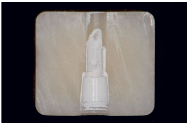
Fig 4 Cross section of lithium-disilicate (LS2) glass-ceramic block after pull-off test.
