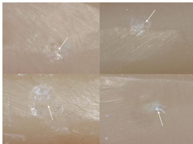
**Fig 4** Deterioration features produced by the mechanical compressive cyclic loading (Biocycle V2) in four different specimens: minor signs of wear and contact damage (arrows) limited to the area in contact with the load piston were observed, exhibiting a typical pattern of localized rough surface. These surface deterioration features were not considered compatible with signs of deterioration observed in vivo.
