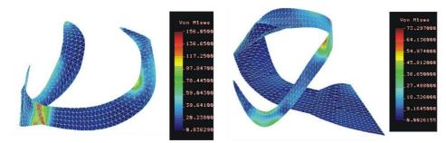
Fig. 7. Equivalent stress distribution when static (20N) and thermal charges (0°C) were cumulated: a) Akers clasp. b) back action clasp.
