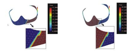
Fig. 3. Temperature distribution for the Akers Fig. 4. Temperature distribution for the back clasp in case of thermal variations from 37°C action clasp in case of thermal variations from 37°C to 60°C. to 0°C.
