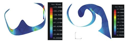
Fig. 1. Von Misses equivalent stress resulting Fig. 2. Von Misses equivalent stress resulting the simulation of a static charge (average force of 20N) in the Akers clasp.
