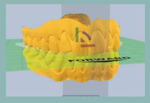
**Fig 5-1-7** Model preparation module of Archform, showing the different planes used for model orientation with the option to tilt/translate the model in relation to these planes.
