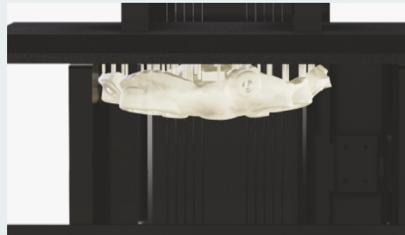
1-17. Surgical guide is fabricated using a 3D printer.
