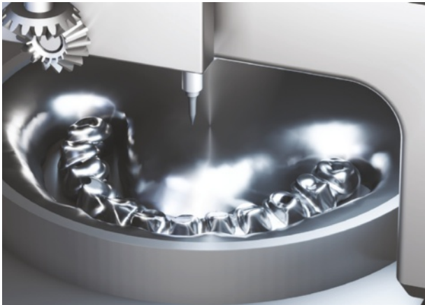
1-36. Titanium framework is fabricated using the CAD-CAM milling process.
