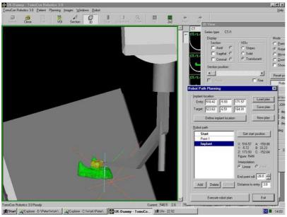
Controlling the plan before drilling
