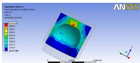
Fig. 6: Stresses in the female insert
