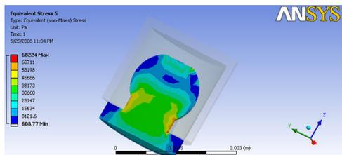
Fig. 8: Stresses in the metal ball
