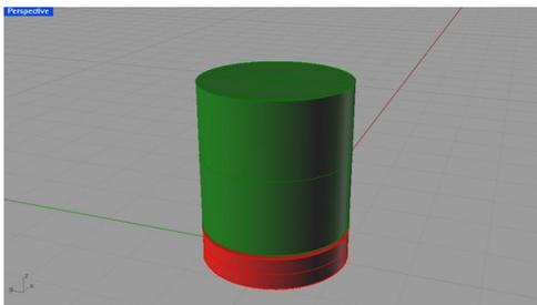
Fig. 3: Modeling of the resilient female insert
