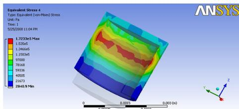
Fig. 9: Stresses in the metal housing
