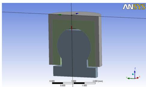
Fig. 5: Section through a resilient ball and socket stud type attachment
