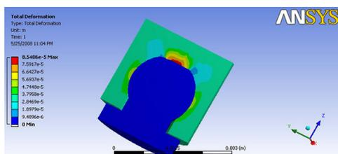
Fig. 7: Displacements in the female insert
